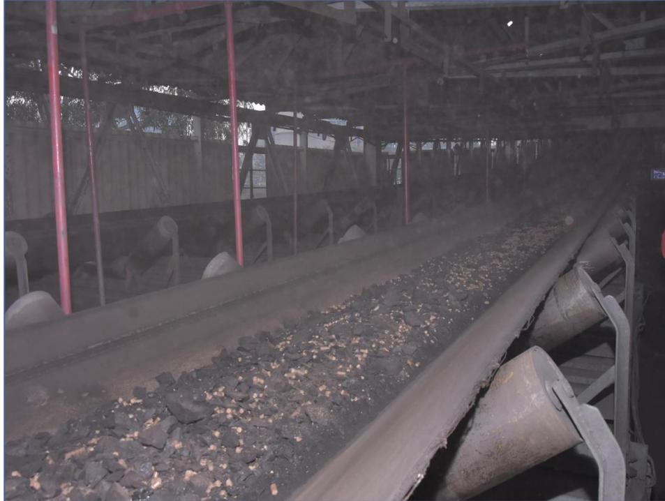
**Blended Biomass Pellets fed to Boiler**
